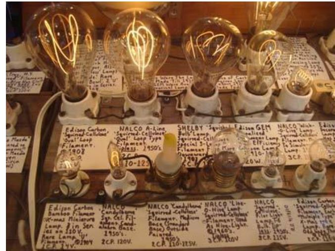
Among numerous experiments, Edison's team finally discovered that carbonized bamboo filament could last over 1,200 hours.
